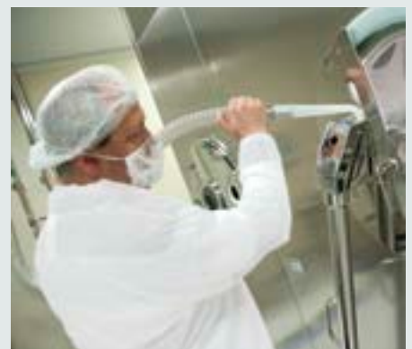
Cleaning of a coating pan
