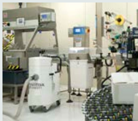
Recovery of waste from a packaging machine
