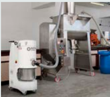
Daily cleaning of driers
