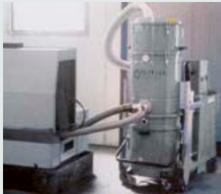
Fixed application for recovery of graphite
