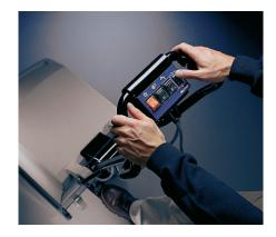
Simple, clearly marked controls are within easy reach of the user. Convenient foot pedal raises and lowers brush. The adjustable handle adapts to fit any person
