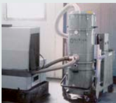
Fixed application for recovery of graphite
